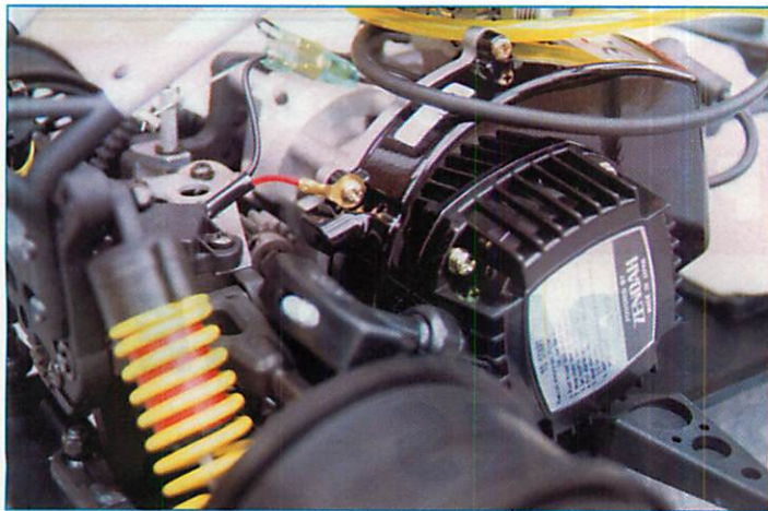
Above left: 22.5 Zenoah 2 stroke motor with pull starter.
