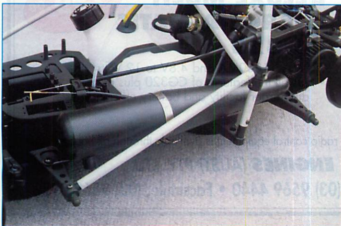
Below: Tuned pipes helps the Zenoah engine. Comes as standard.
